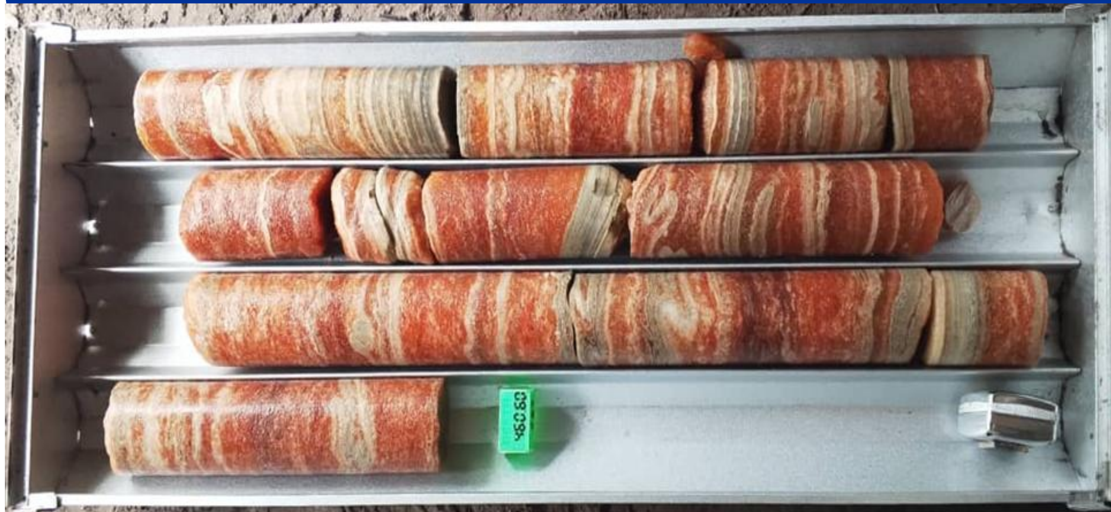
Red Carnallite-rich core from BA_004 showing interbedded banded and nodular Carnallite with banded Halite at approx. 458m to 461m depth
