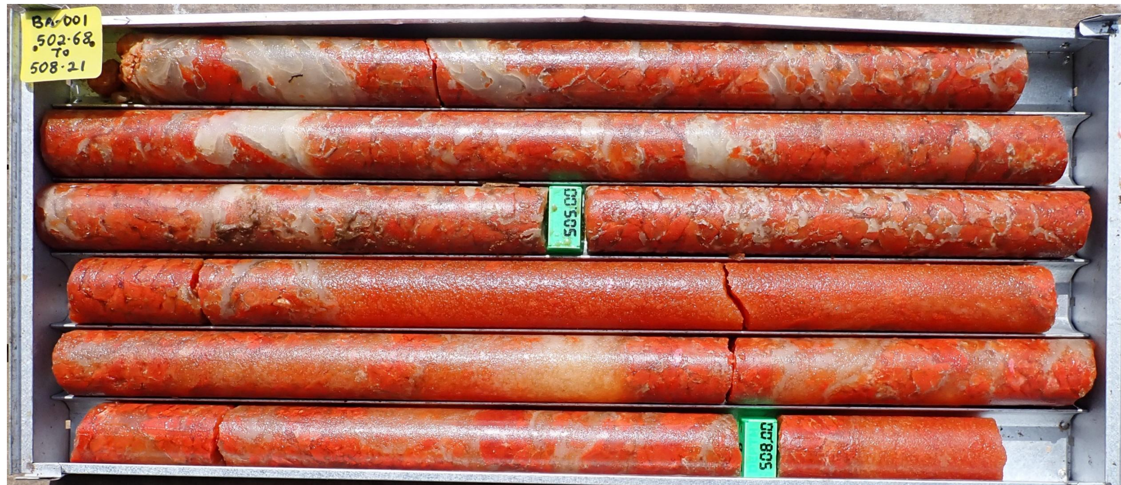
Hole BA-001-EXT Red carnallite interbedded with halite, depth of approx. 503m-508m
