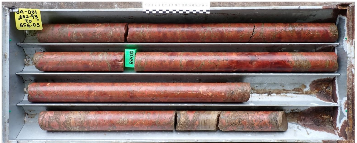
Photo 2 Red Carnallite-rich core from BA-001-EXT with massive nodular Carnallite and bedded Halite at approx. 653m to 656m depth
