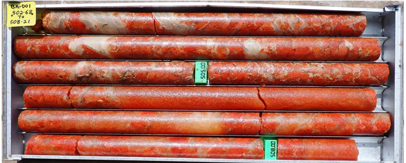
Photo 1 Red Carnallite-rich core from BA_001-EXT showing interbedded nodular Carnallite and Halite with soft sediment deformation features at approx. 503m to 508m depth
