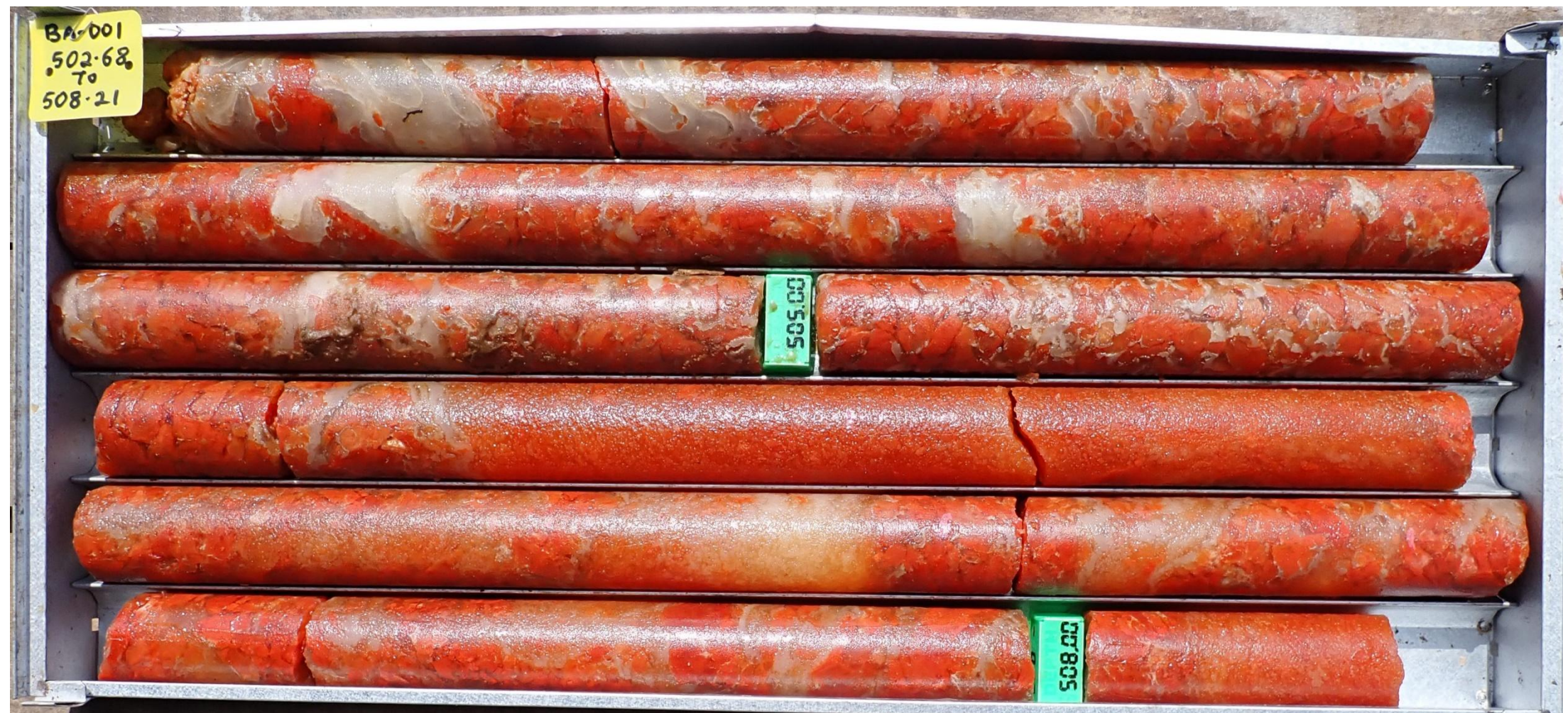
Hole BA-001-EXT Red carnallite interbedded with halite, depth of approx. 503m-508m
