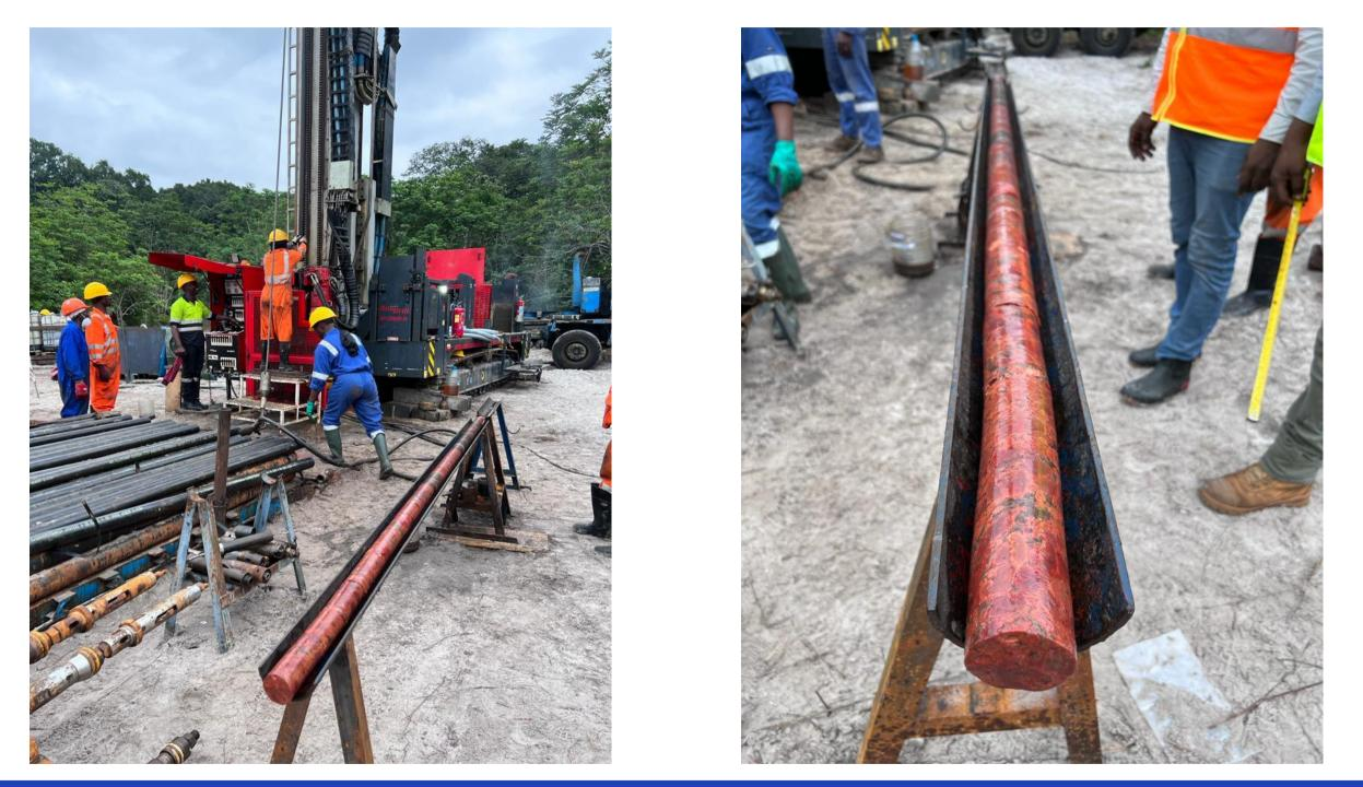
Stage 1 drill program began with the extension of historic drillhole BA-002 with coring beyond the bottom of the old hole to a depth of 552.5m. Potash mineralization, in the form of bright red nodular carnallite bedding was intersected from Cycle IV & Cycle III evaporite sequence.
