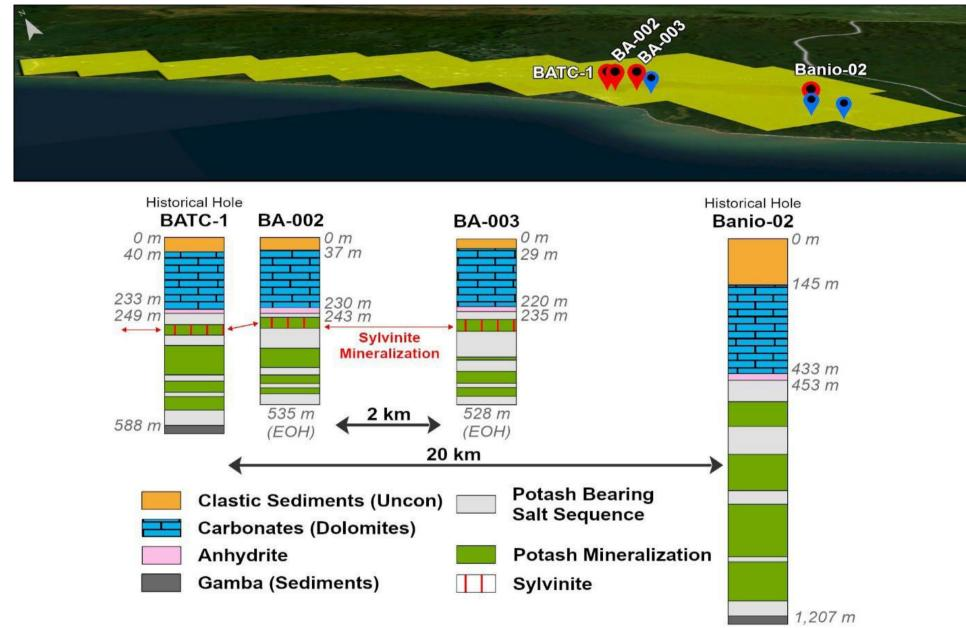
Previously drilled holes in red at Banio. Good correlation of potash cycles between holes BA-002 and BA-003 and with oil/gas holes BATC-1 and BA-002 located 20 km south within the license.
