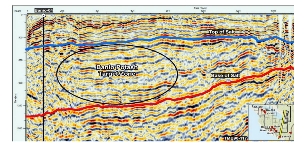
Reinterpretation of historic seismic data identifies potash bearing Salt Sequence up to 800m thick with potential to host multiple carnallitite and sylvinite horizons.
