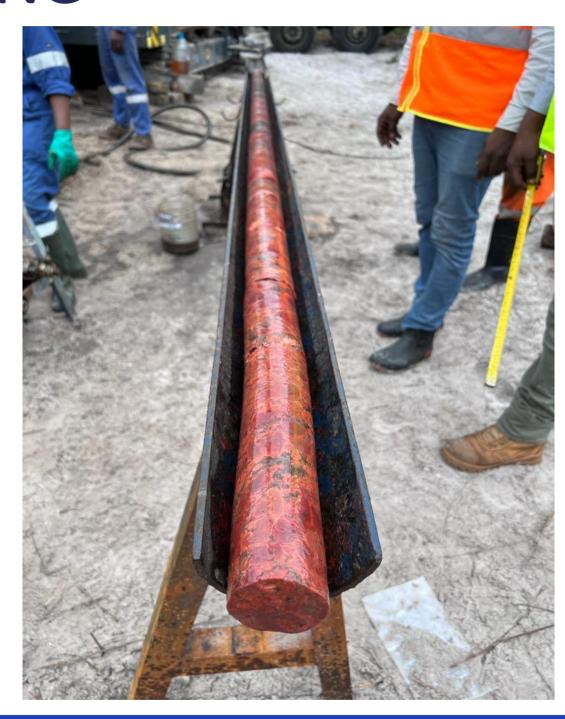
Stage 1 drill program focused on the extension of historic drillhole BA002 with coring beyond the bottom of the old hole at a depth of approx. 519m
