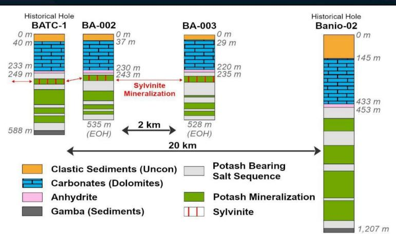
Previously drilled holes in red at Banio. Good correlation of potash cycles between holes BA002 and BA003 and with oil/gas holes BATC-1 and B02 located 20 km south within the licence.
