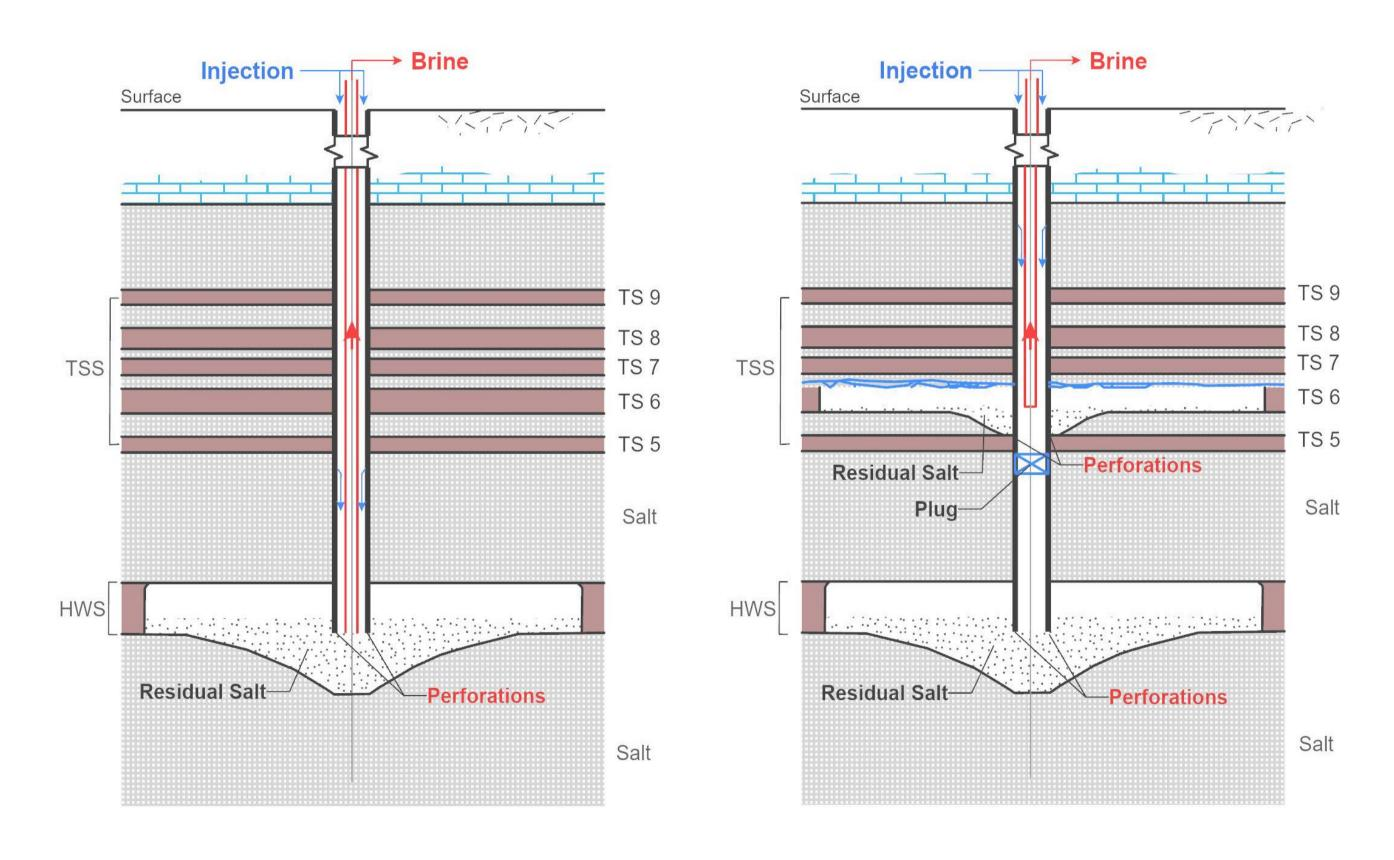
Solution mining potential; several potash-bearing layers can be exploited using single well injection/extraction. Solution mining typically has lower CAPEX than conventional U/G mining and can be carried out in stages with a modular approach
