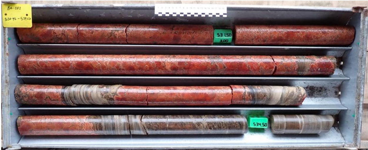
Fig. 3 Potash mineralization in drill core from BA-002 Extension showing nodular red carnallite with banded bedded halite attributed to Cycle III.
