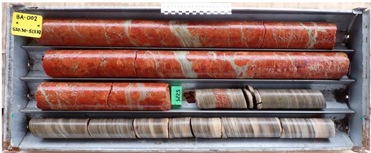
Fig. 2 Potash mineralization in drill core from BA-002 Extension showing nodular red carnallite and laminated halite attributed to Cycle IV (Hole Dip=90°).
